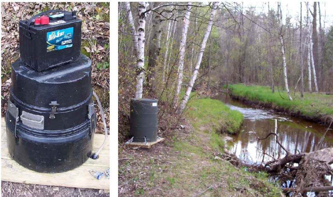
Figure 3.2. (a) ISCO Model 1392 Wastewater Sampler and (b) view of the North Branch sampling site showing sampler and staff gage.
