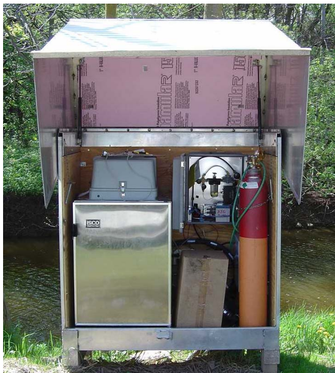
Figure 3.4. Automated USGS monitoring station with ISCO 3700R sampler, gas bubbler, and data logger.
