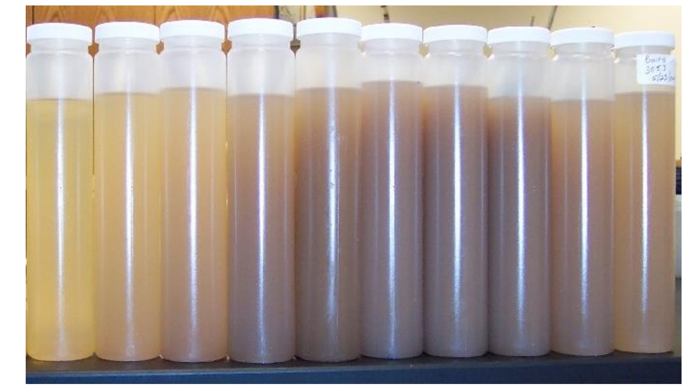
Figure X. Samples showing sediment concentration change over a storm.
