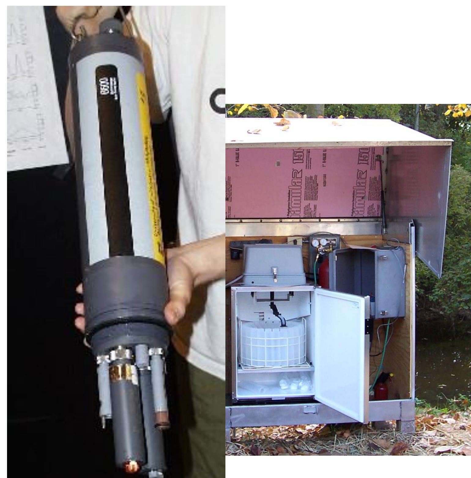
Figure X. YSI-6200 multi-parameter sonde. Refrigerated ISCO sampler.
